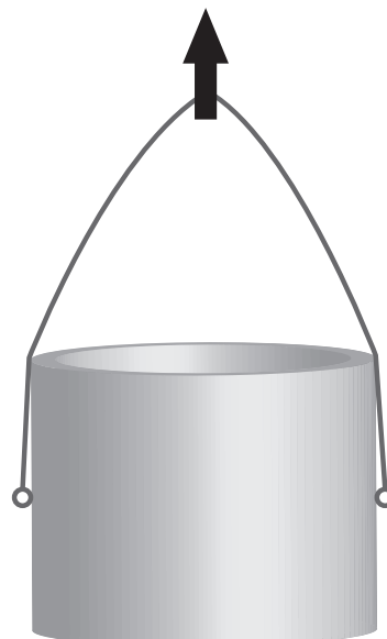
ACCEPTABLE LIFTING METHOD
